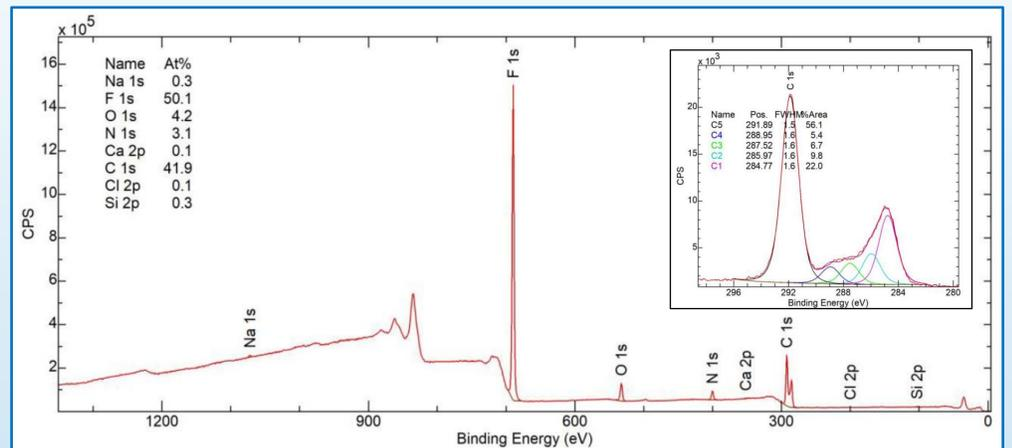
Surface analytics by XPS provides quantitative information about elemental composition within 2 nm to 10 nm; deconvolution of high-resolution spectra delivers information about oxidation and binding state. Determination of all elements except H and He: C/F/O/Si/N/P/Na/Ca/S etc. C-C/C-H vs. C-O vs. C=O vs. COOR vs. CF<sub>3</sub>. F: covalent vs. ionic.
